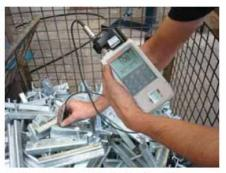
Electronic gauge for galvanize coating thickness check
