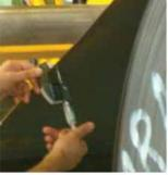
Digital micrometer for material thickness check
